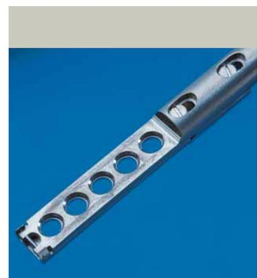
Multiple specimen holder for TEM specimens
